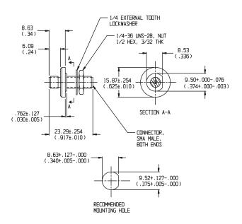
NOTE: All dimensions are given in mm (inches) and are maximum, unless otherwise specified.
