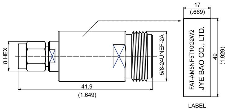
Nominal impedance: 50Ω±0.25Ω over operating temperature range.
