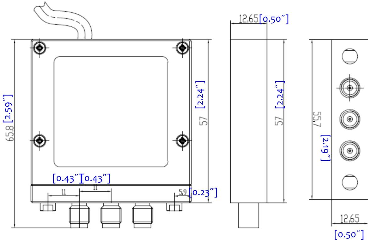
SPDT Absorptive Electro-Mechanical Switch DC-40GHz
