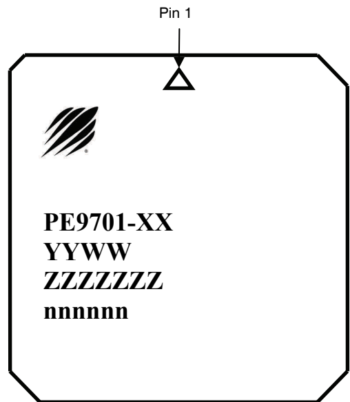
Figure 8. Top Marking Specifications
