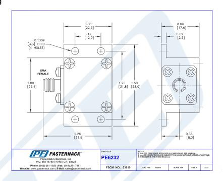
Medium Power 50 Watts RF Load Up To 3 GHz With SMA Female Input Square Body Nickel Plated Brass from Pasternack Enterprises has same day shipment for domestic and International orders. Our RF, microwave and millimeter wave products maintain a 99% availability and are part of the broadest selection in the industry.
