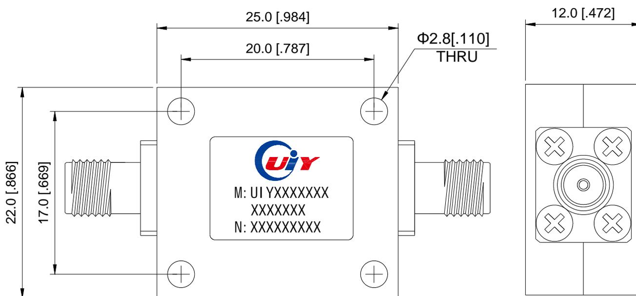
Unit: mm/ inch, General part tolerance is  $\pm 0.2$ mm unless otherwise stated.
