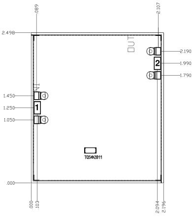
Unit: millimeters Thickness: 0.10 Die x, y size tolerance:  $\pm 0.050$ Chip edge to bond pad dimensions are shown to center of pad Ground is backside of die
