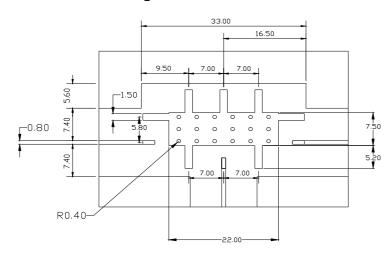
NOTE: SUBSTRATE IS 1.6MM THICK FR4 WITH GND PATTERN UNDER UNIT ON TOP LAYER CONNECTED TO FULL GND PLANE ON BOTTOM LAYER
