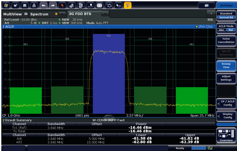
Adjacent channel leakage ratio (ACLR) measurement of a 3GPP WCDMA signal.
