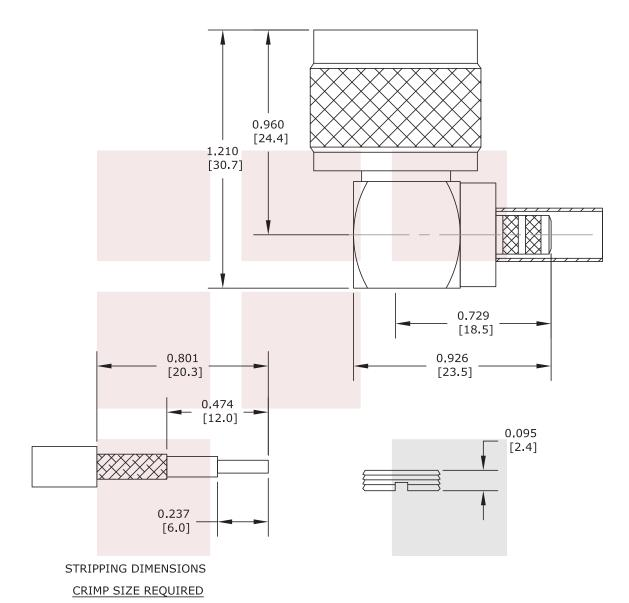
CONTACT PIN: SOLDER FERRULE: .213" HEX CRIMP TOOL
