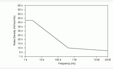
Representation of NI 5122 Spectral Noise Density on 0.2 V Range, Full Bandwidth, 50  $\,\Omega$  Input Impedance
