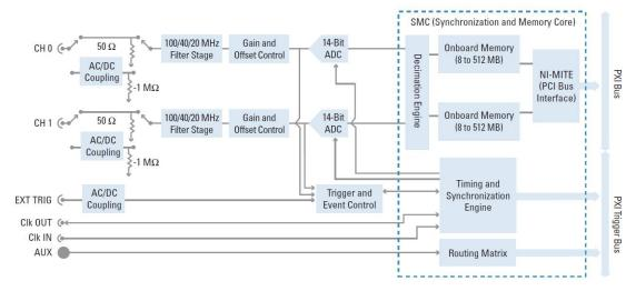
Figure 2. Hardware Block Diagram
