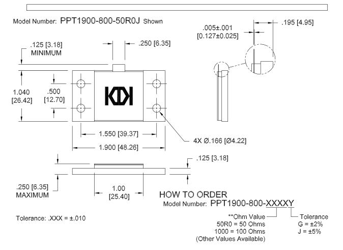
Note: Dimensions in Brackets are Expressed in Millimeters and are for Reference Only. Design Specifications are subject to change without notice.
