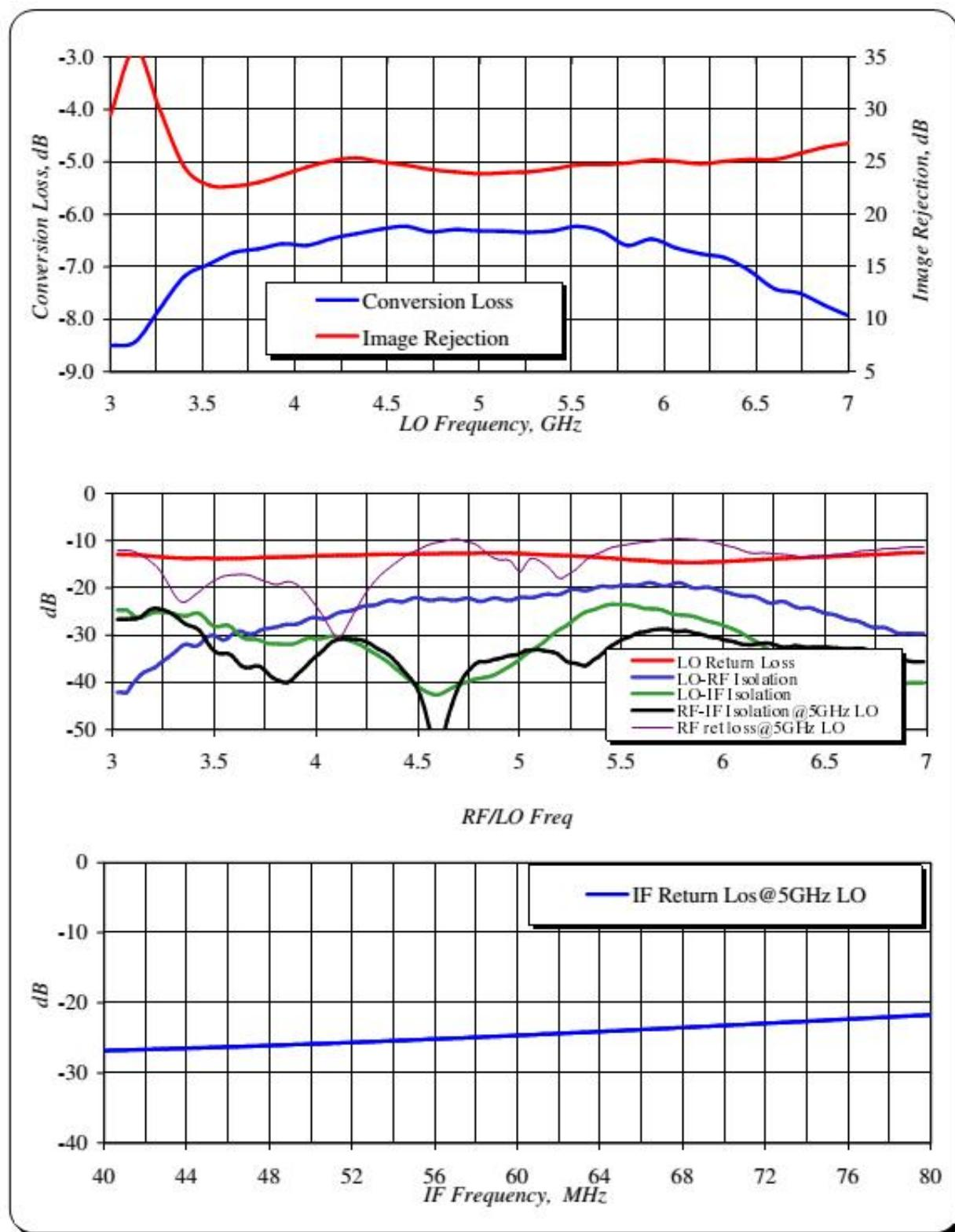
Typical measured data @ 25C with LO power = +5 dBm
