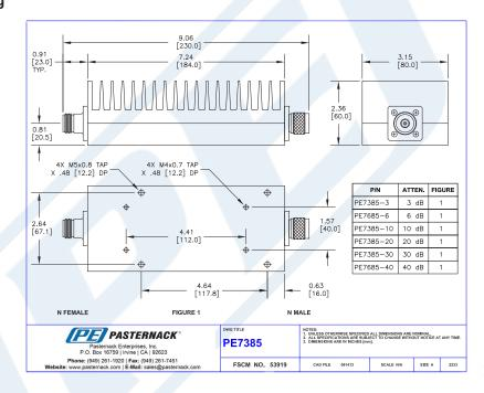
40 dB Fixed Attenuator, N Male To N Female Black Anodized Aluminum Heatsink Body Rated To 100 Watts Up To 3 GHz from Pasternack Enterprises has same day shipment for domestic and International orders. Our RF, microwave and millimeter wave products maintain a 99% availability and are part of the broadest selection in the industry.
