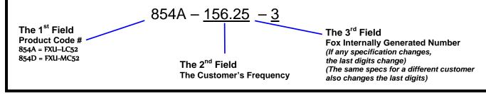
This example, FXU-LC525R-156.25 = LVDS Output, Ceramic,  $5 \times 3.2$ mm Package, 2.5V,  $\pm 50$  PPM Stability, -40 to +85°C Temperature Range, at 156.25 MHz
