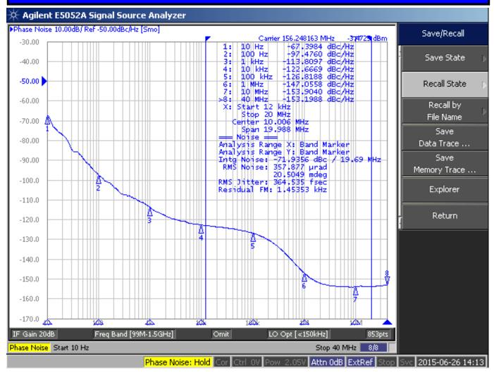
Jitter is frequency dependent. Below are typical measured values for 156.25 MHz. (Consult Fox Tech Support for other frequencies.)
