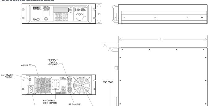
RF OUTPUT (WAVEGUIDE FLANGE) Ku-BAND-WR-75
