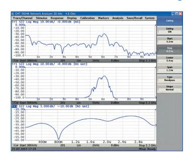
This function mathematically removes unwanted responses in the time domain, which allows the user to obtain frequency response without influence from fixture elements.
