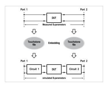
This function allows the user to mathematically simulate DUT parameters by virtually integrating a fixture circuit between the calibration plane and the DUT. This circuit should be described by an S-parameter matrix in a Touchstone file.
