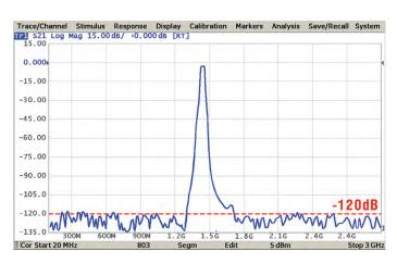
Typical dynamic range of 123 dB is achieved through the entire frequency range (at 1 Hz IF bandwidth). Seen here is the maximum dynamic range achieved when using IFBW 1 Hz and an output power level of 10 dBm.
