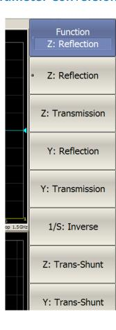
The function allows conversion of the measured S-parameters to the following parameters: reflection impedance and admittance, transmission impedance and admittance, and inverse S-parameters.
