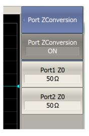
This function converts the S-parameters measured at the 75  $\Omega$  port into values, which could be determined if measured at a test port with arbitrary impedance.
