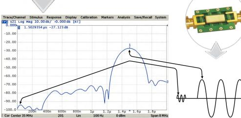
This function performs data transformation from frequency domain into response of the DUT to various stimulus types in time domain. Modeled stimulus types: bandpass, lowpass impulse, and lowpass step. Time domain span is set by the user arbitrarily from zero to maximum, which is determined by the frequency step. Windows of various forms are used for better tradeoff between resolution and level of spurious sidelobes.
