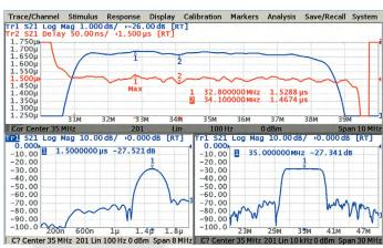
Time domain analysis allows measurement of parameters of SAW filters such as the signal time delay, feedthrough signal suppression.
