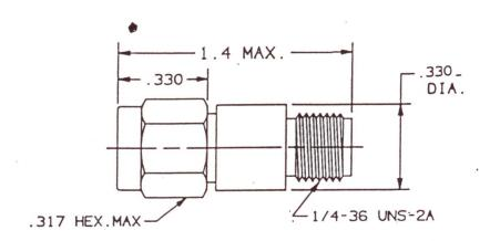
D.C. Blocks are generally used to prevent D.C. voltages from damaging susceptible RF circuitry. The units cover a range from below 1 MHz to a minimum of 10 GHz. Low insertion loss and good VSWR are features of these units.
