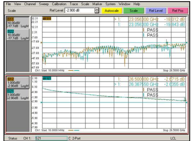
Test #1: SMA Male to SMA Male, 24 inches, DC - 26.5 GHz
