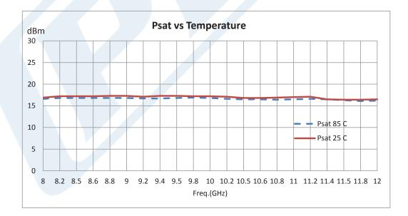
Click the following link (or enter part number in "SEARCH" on website) to obtain additional part information including price, inventory and certifications: 2.2 dB NF, 20 mW, 8 GHz to 12 GHz, Low Noise Amplifier, 38 dB Gain, SMA PE15A1003
