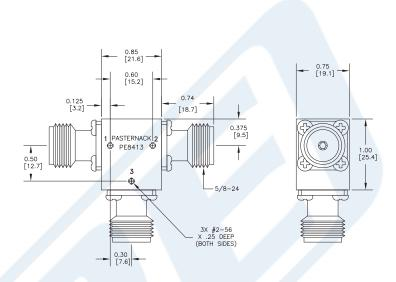
50 Ohm N Circulator Operating From 7 GHz to 12.4 GHz And 10 Watts With 20 dB Isolation from Pasternack Enterprises has same day shipment for domestic and International orders. Our RF, microwave and fiber optic products maintain a 99% availability and are part of the broadest selection in the industry.
