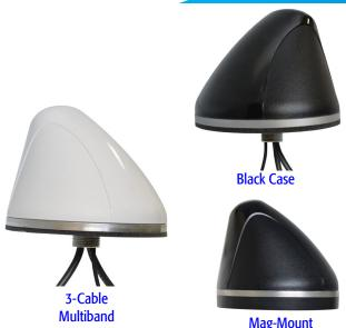
The SMW-308 Series Antenna features 3-elements in one antenna radome. The unique feature of this SMW model is that it offers two elements covering US Cellular frequencies. The first cellular element is the broadband element found in other SMW antennas and covers 800-1250 & 1650-2700 MHz. The second element, because it is shorter, covers 824-894 & 1850-1990 MHz.
