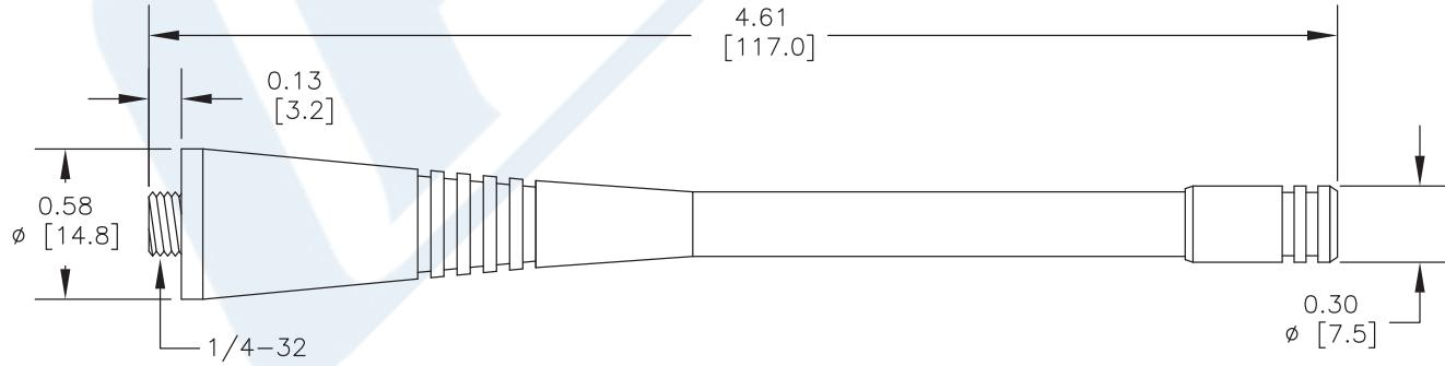
Click the following link (or enter part number in "SEARCH" on website) to obtain additional part information including price, inventory and certifications: [Whip Antenna Operates From 482 MHz to 512 MHz With a Typical 0 dBi Gain MX Input Connector IP67 Rated PE51147](#)
