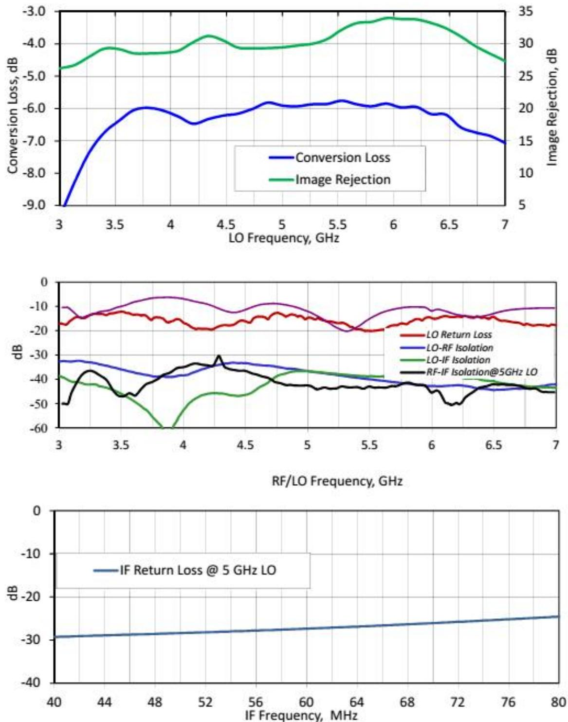
Typical measured data @ 25C with LO power = +15 dBm
