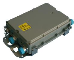
CCI's Twin TMA contains two TMAs in a single housing. Each TMA is full band and fully duplexed. High linearity improves the uplink sensitivity and the receive performance of base stations.
