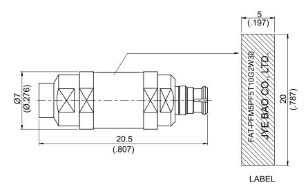
Nominal impedance:  $50\Omega$ +/-0.25 $\Omega$  over operating temperature range. Operating temperature range: -50 degrees Celcius to +80 degrees Celcius.
