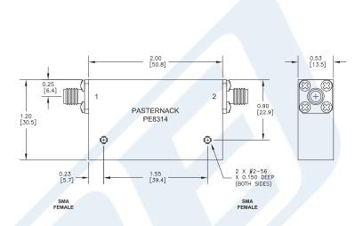
50 Ohm SMA Isolator Operating From 3.5 GHz to 12.8 GHz And 2 Watts With 17 dB Isolation from Pasternack Enterprises has same day shipment for domestic and International orders. Our RF, microwave and fiber optic products maintain a 99% availability and are part of the broadest selection in the industry.
