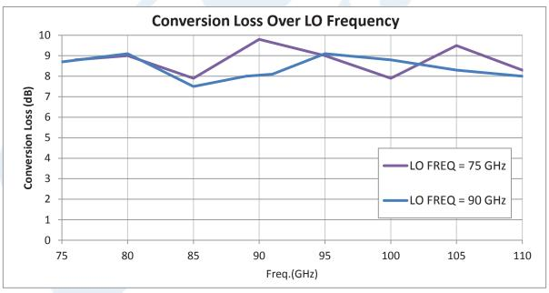
Click the following link (or enter part number in "SEARCH" on website) to obtain additional part information including price, inventory and certifications: Waveguide Mixer Up Converter WR-10 From 75 GHz to 110 GHz, IF From DC to 18 GHz And LO Power of +13 dBm, UG-387/U Flange, W Band PE13U1000
