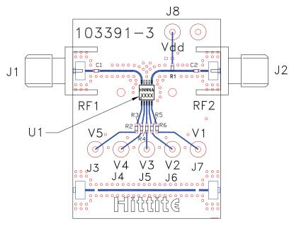
\* R2 - R6= 100 Ohm. These resistors are optional and may be used to enhance decoupling of the RF path from the control inputs.
