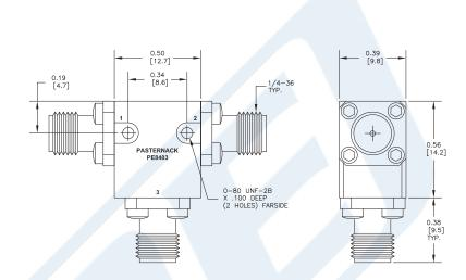
50 Ohm SMA Circulator Operating From 7 GHz to 12.4 GHz And 10 Watts With 18 dB Isolation from Pasternack Enterprises has same day shipment for domestic and International orders. Our RF, microwave and fiber optic products maintain a 99% availability and are part of the broadest selection in the industry.
