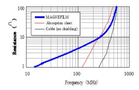
By mounting MAGNEFILM on both sides of FPC (length=10cm), higher loss effect can be obtained in low-frequency band, compared to absorption sheet (MG-02 t=0.1).
