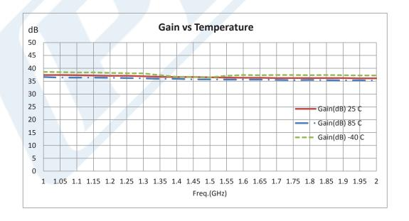
Click the following link (or enter part number in "SEARCH" on website) to obtain additional part information including price, inventory and certifications: 1.5 dB NF, 10 mW, 1 GHz to 2 GHz, Low Noise Amplifier, 35 dB Gain, SMA PE15A1000
