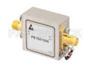
1.5 dB NF, 10 mW, 1 GHz to 2 GHz, Low Noise Amplifier, 35 dB Gain, SMA
