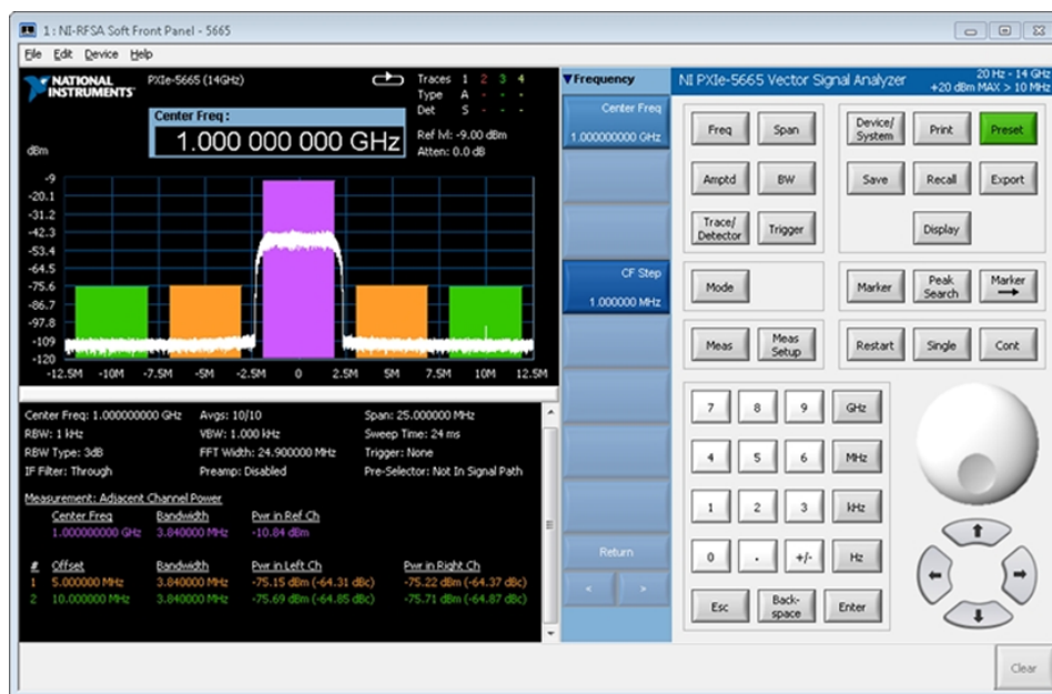
Figure 11. NI-RFSA SFP Showing an ACP Measurement
