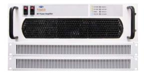
The BT-AlphaS series is a range of class AB RF power amplifiers covering the 100kHz to 30MHz frequency range
