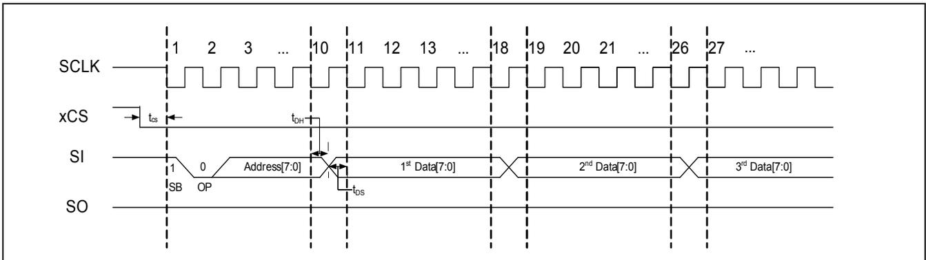
**Figure 4-6. 4-wire Random READ Timing Diagram**
