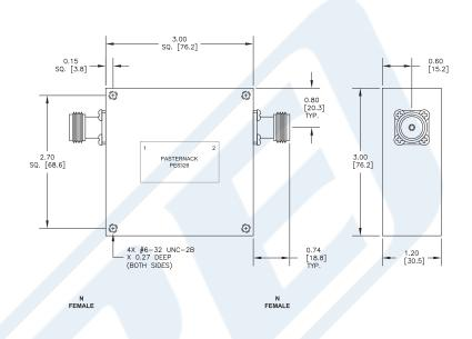
50 Ohm N Isolator Operating From 450 MHz to 520 MHz And 150 Watts With 20 dB Isolation from Pasternack Enterprises has same day shipment for domestic and International orders. Our RF, microwave and millimeter wave products maintain a 99% availability and are part of the broadest selection in the industry.
