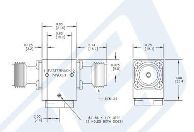
50 Ohm N Isolator Operating From 7 GHz to 12.4 GHz And 10 Watts With 20 dB Isolation from Pasternack Enterprises has same day shipment for domestic and International orders. Our RF, microwave and fiber optic products maintain a 99% availability and are part of the broadest selection in the industry.
