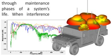
EMIT will combine antenna isolation from antenna simulation tools and measurements when available.
