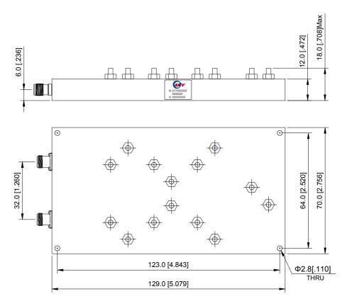
Unit: mm/ inch, General part tolerance is ±0.2mm unless otherwise stated.
