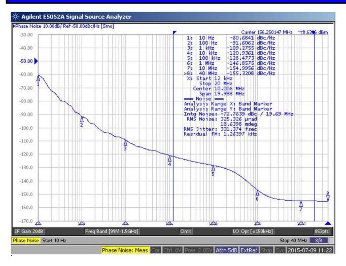
Jitter is frequency dependent. Below are typical values at 156.25 MHz.
