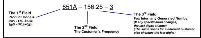
This example, FXU-HC525R-156.25 = HCMOS Output, Ceramic,  $5 \times 3.2$ mm Package,  $2.5 \times 50$  PPM Stability,  $-40 \times 60 \times 10^{-2}$  to  $+85 \times 60 \times 10^{-2}$  C Temperature Range, at 156.25 MHz
