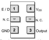
Terminations as viewed from the Top NOTE: XPRESSO-Ultra HCMOS XOs are designed to fit on Industry Standard, 4 pad layouts
