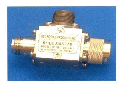
The FTP-14BH Bias Tap is used to provide a DC path to one side of a 50 Ohm transmission line. An integral blocking capacitor isolates the DC from the other side of the line.
