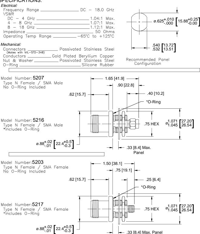
Panel Nut, Lock Washer and O-Ring are Shipped Unassembled.
