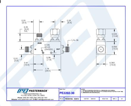
Directional 30 dB SMA Coupler From 2 GHz to 4 GHz Rated To 50 Watts from Pasternack Enterprises has same day shipment for domestic and International orders. Our RF, microwave and millimeter wave products maintain a 99% availability and are part of the broadest selection in the industry.
