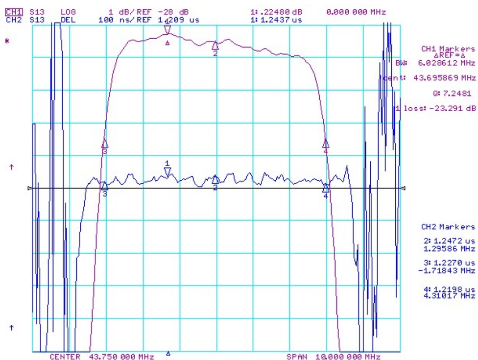
Figure-2 S21 Response(Pass Band/Span=10MHz)
