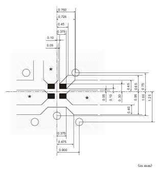
\*Line width to be designed to match 50  $\Omega$  characteristic impedance, depending on PCB material and thickness.
