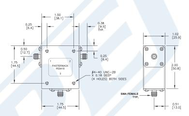
50 Ohm SMA Circulator Operating From 698 MHz to 960 MHz And 1000 Watts With 18 dB Isolation from Pasternack Enterprises has same day shipment for domestic and International orders. Our RF, microwave and fiber optic products maintain a 99% availability and are part of the broadest selection in the industry.
