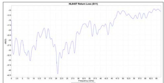
Figure 5: Typical return loss on RF In port of the HL9407
