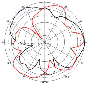
Freq:2450MHz Date:2014-10-31 Elevation:V-plane Polar-Across:Main Polarization:Vertical Max:-38.77dB HPBW(3dB):74.92\* FBR:1.52dB Obliquity:27.45\*
