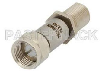
DC Block on Inner Conductor 75 Ohm F Male to F Female Operating From 10 MHz to 2 GHz
