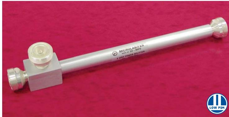
Microlab Model Dx-85FD series of 2, 3 and 4 way Power Splitters has been designed to evenly split high power cellular signals with minimal reflections and loss. Joints are moisture sealed with gaskets to meet IP67. The rugged, lightweight design can be easily attached to a wall with the supplied bracket and clip.
